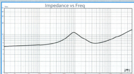
FIGURE 1: Morel ST 1108 free-air impedance plot.
